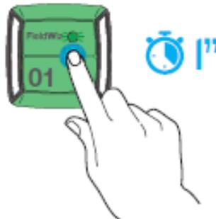
It is required for the proper functioning of the device to check the position on each player and that the LED is pulsing (In the right position you can read the number and see the LED pulsing)
